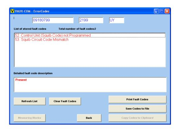
You can see from the Fault Code list, that the Airbag ECU needs to be programmed.
