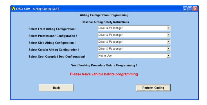
When you selected the proper configuration, please click on the [Perform Coding] button, to perform the programming of the Airbag ECU.
